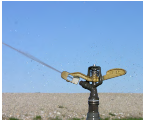
Inspect the sprinkler nozzles yearly. Measure the opening of the nozzle to check if it is worn down. If it is out of tolerance, replace it.
