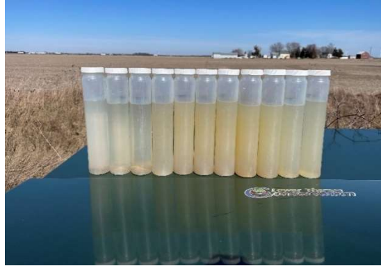
Figure 4. Visual assessment of variations in water quality following a sampling event, demonstrating baseline [Left], rising flow [Middle Left], peak flow [Middle], and descending limb of flow [Right].
