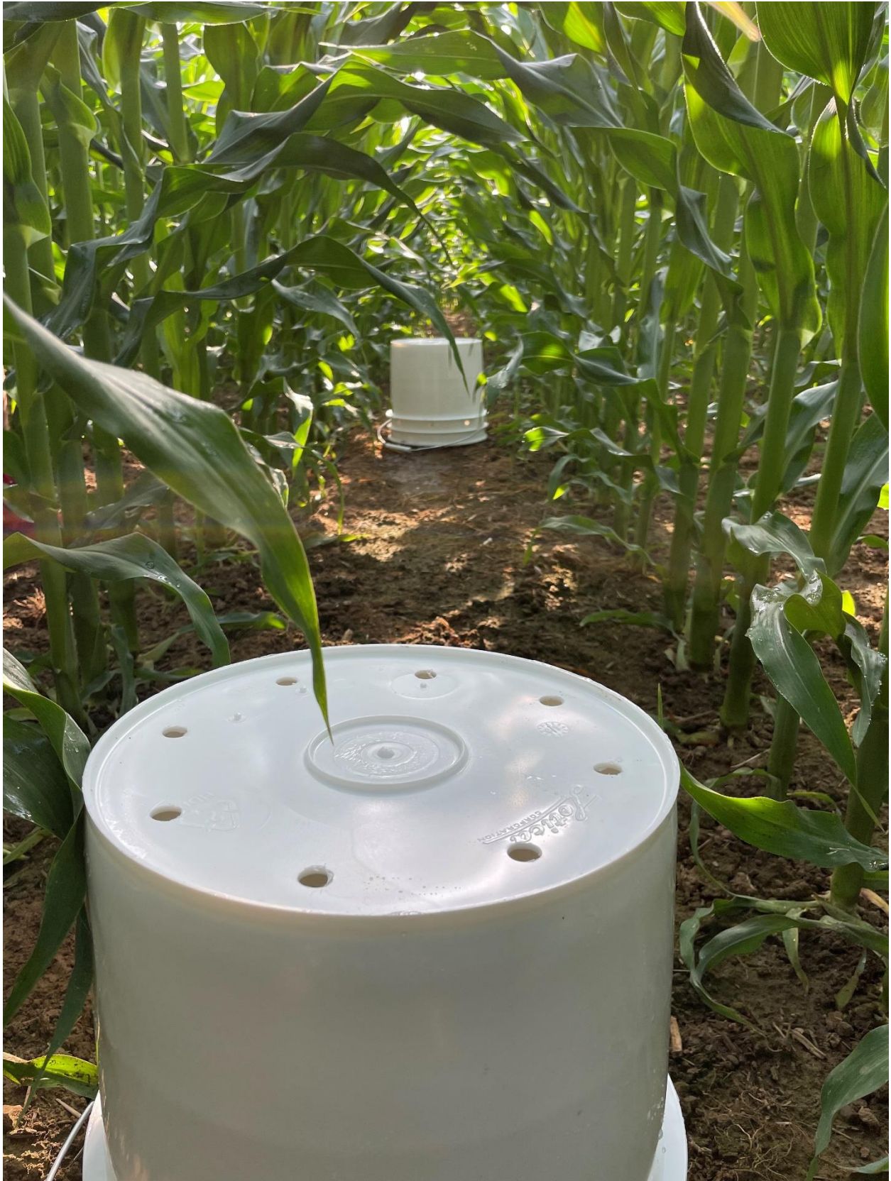
Example of dosimeter location configuration for late application of ammonia in corn
