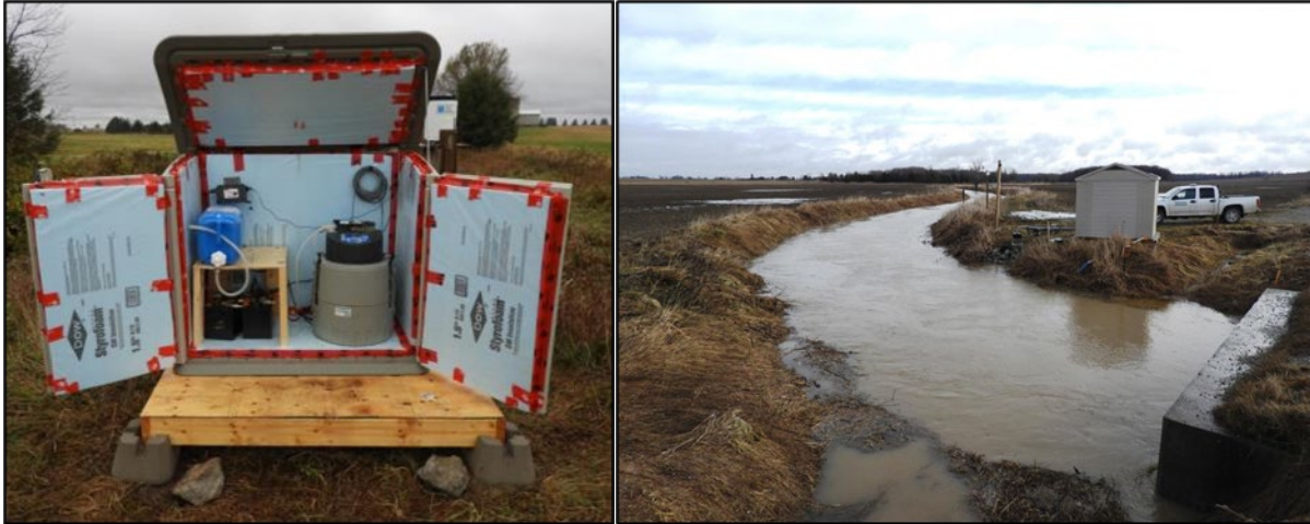
Figure 32. The inside of a water monitoring station established by UTRCA (left) and a watershed monitoring station during a period of high-flow.
