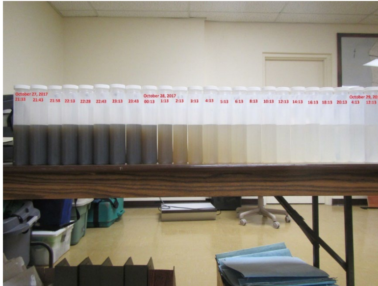
Figure 24. Photograph of tile water samples collected from the Garvey Glenn EOF site during the Oct 27 th event.
