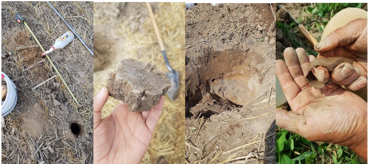
Figure 3. Photos of soil characterization, auger and pit investigations to determine presence and level of degradation
