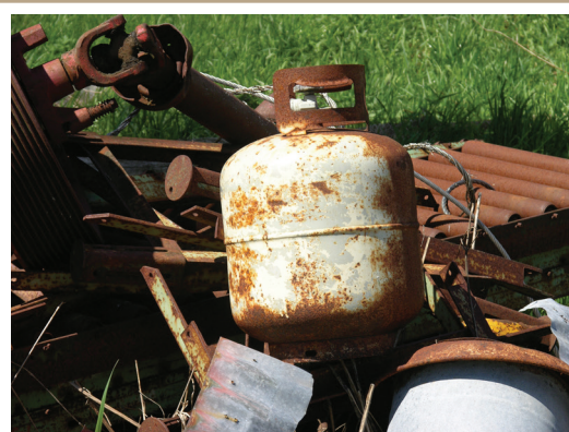
Do not include pressurized containers (e.g. propane tanks) in scrap loads.
