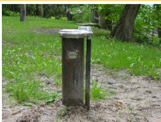
Regrade soil around the well to prevent surface water from ponding near the casing.
