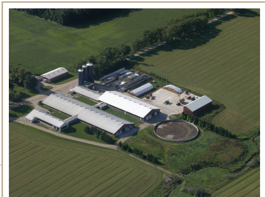
Maximize distance between the ensilage storage and surface water to minimize risk to surface water quality.
