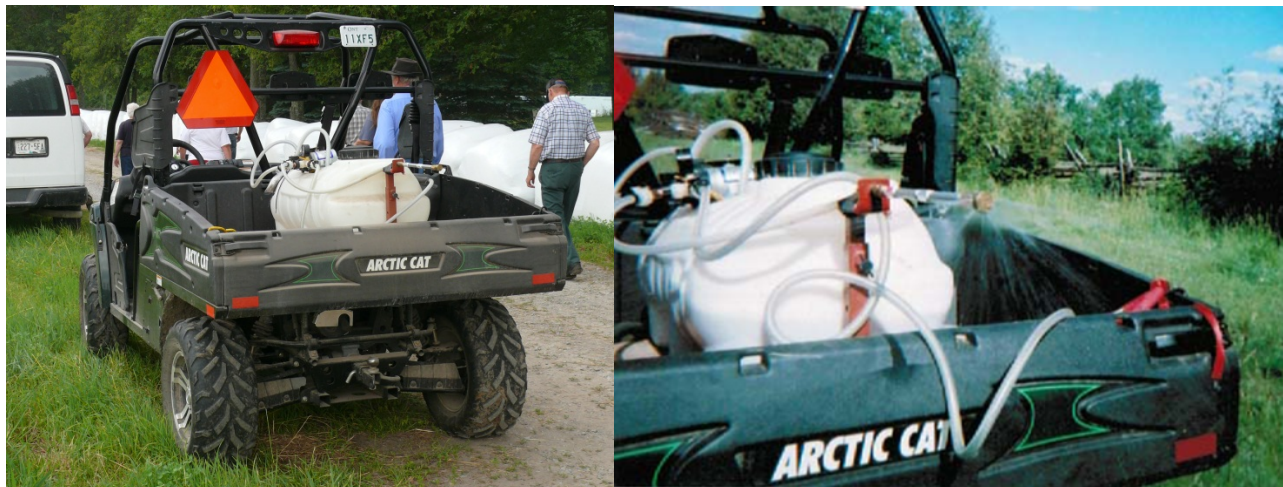
Figure 1. ATV Mounted Sprayer Used in Project
