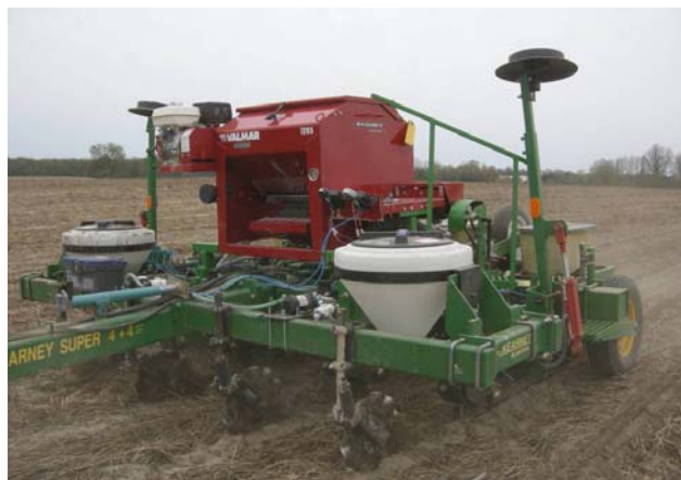
Figure 1. Research planter equipped with liquid and dry starter systems for accurate treatment and rate comparisons.
