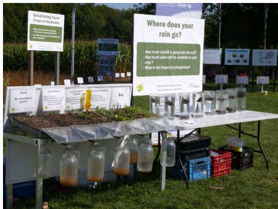
Soil aggregate stability and infiltration is demonstrated for different crop scenarios using rainfall simulator
