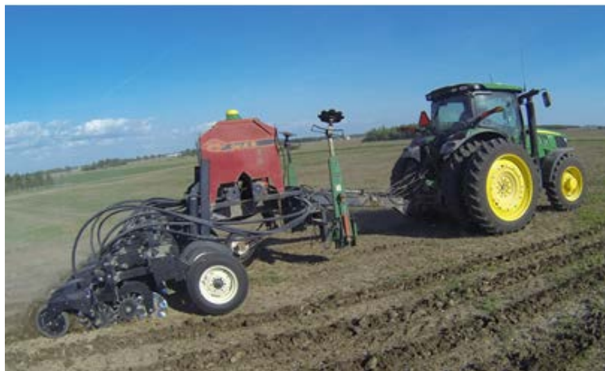
Figure 1. Dawn Pluribus ® strip tiller and Gandy Orbit Air ® dry fertilizer box used to conduct treatments.
