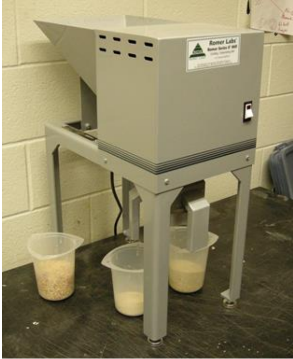
Figure 1. Romer Series II Mill used for simultaneous grinding and subsampling of shelled corn samples.
