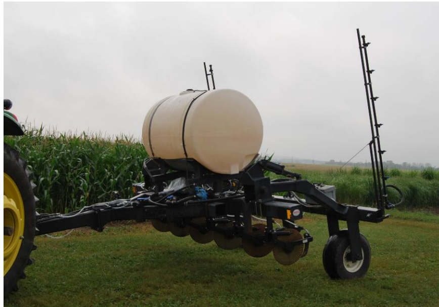
Figure 1. Toolbar with hydraulic UAN pump, knife injectors for sidedressing and steamer nozzle bar for planting time applications.
