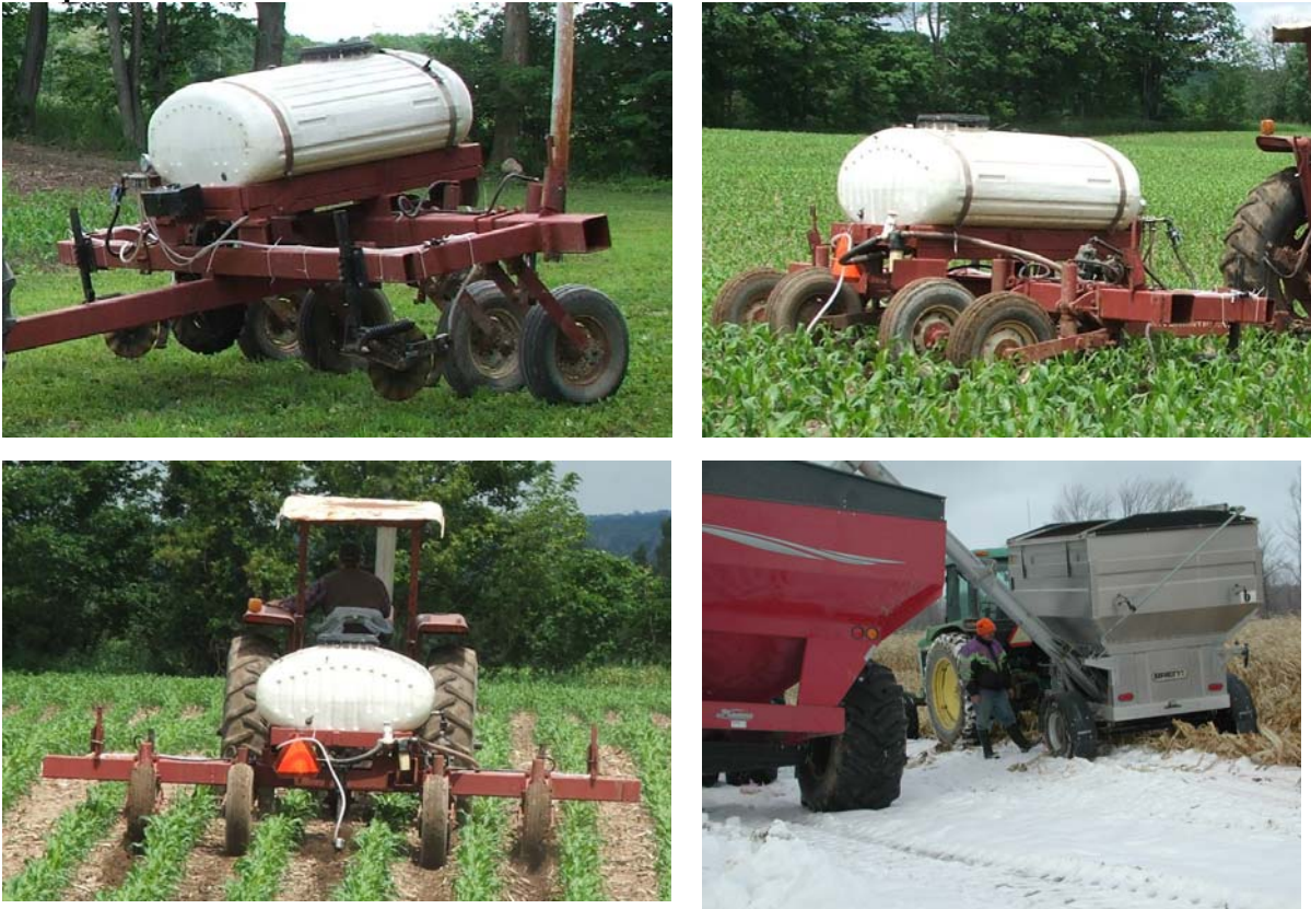
Figure 1. Custom Build Six Row Nitrogen Applicator with Three Fertilizer Coulters Adapted from a Used Corn Planter.
