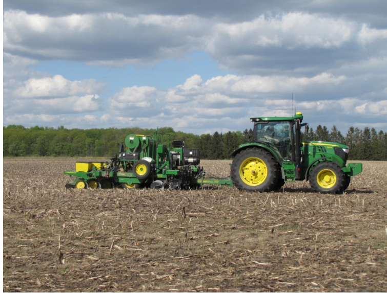
Figure 1. 15 Inch JD Row Unit Precision Planter used in these trials.
