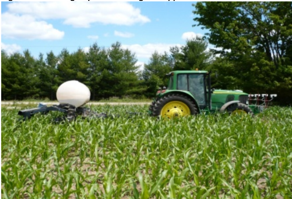
Figure 2. On-the-go optical sensing and application of UAN.
