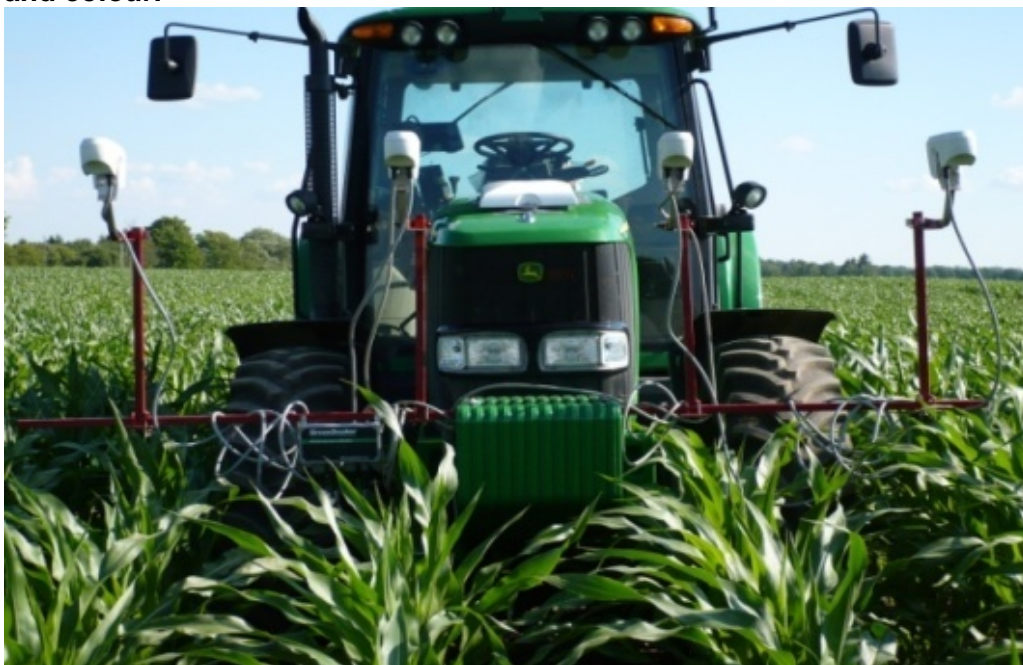
Figure 1. Tractor mounted optical sensors for evaluating corn plant size and colour.
