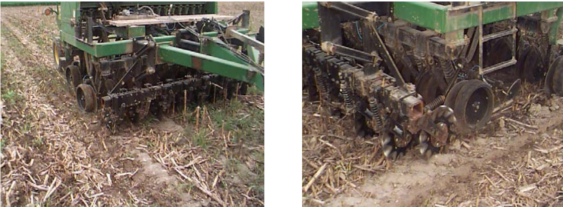
Figure 2. Yetter Coulters Cart attached to a 1560 John Deere Drill
