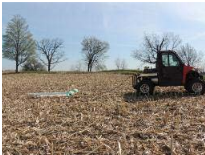
Figure 2. Polaris Ranger pulling Dual EM sensor through corn stubble
