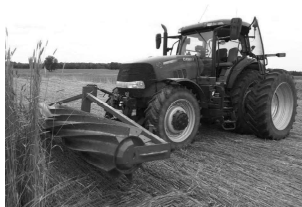
Figure 1. A front-mounted roller crimper being used to terminate cereal rye at anthesis in Ontario, June 2019
