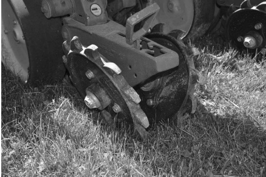
Figure 9. Dawn Gaugetine closing wheels used for seeding soybeans into rye mulch at project sites in 2020.
